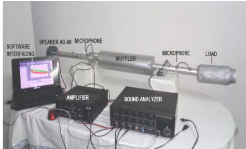
Figure 1: Muffler Transmission loss measurement setup with load
